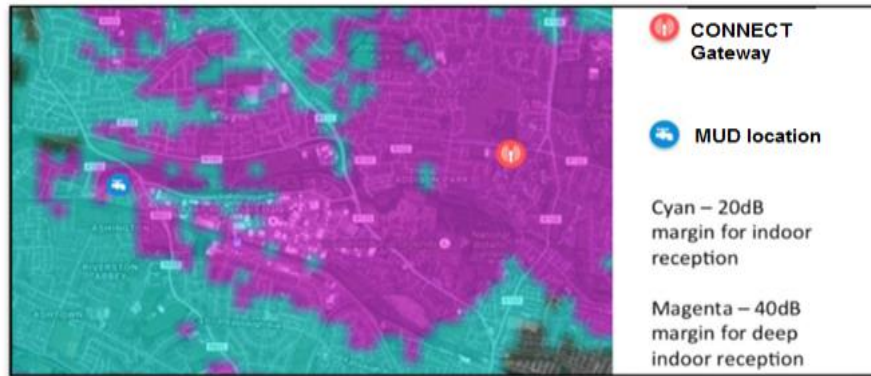
Figure 4: Model of pre-described - LoRA signal strength gateway from the Glasnevin Gateway, around the area of the MUD
