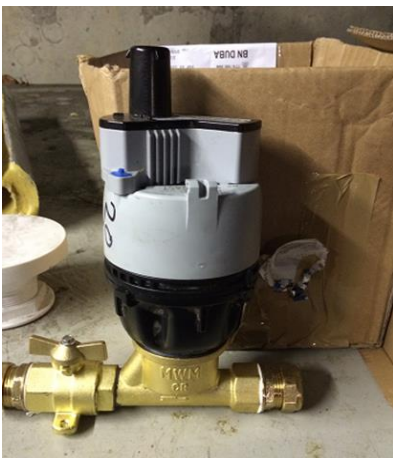
Photo 7: Example of a V210 rotary piston meter with an Ondeo radio
