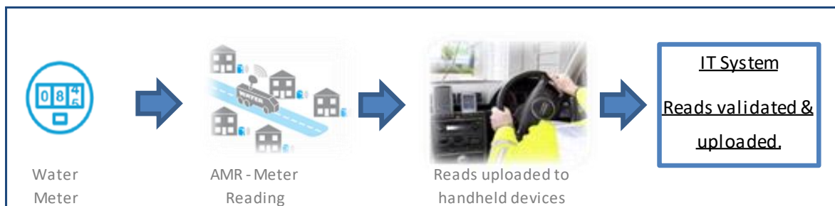
Figure 1: Example of a Meter Reading Technology – Flow diagram
