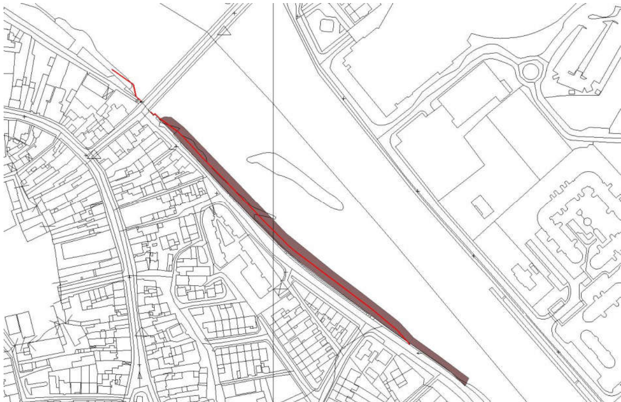
Figure 12 Construction Infill Area that includes for the Temporary haul road
