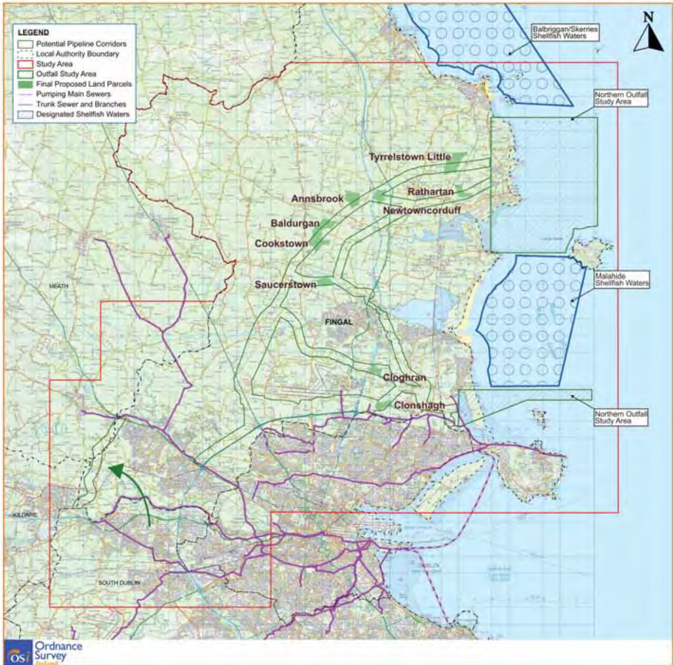
FIG. 2 - POTENTIAL PIPELINE CORRIDORS AND MARINE OUTFALL LOCATIONS
