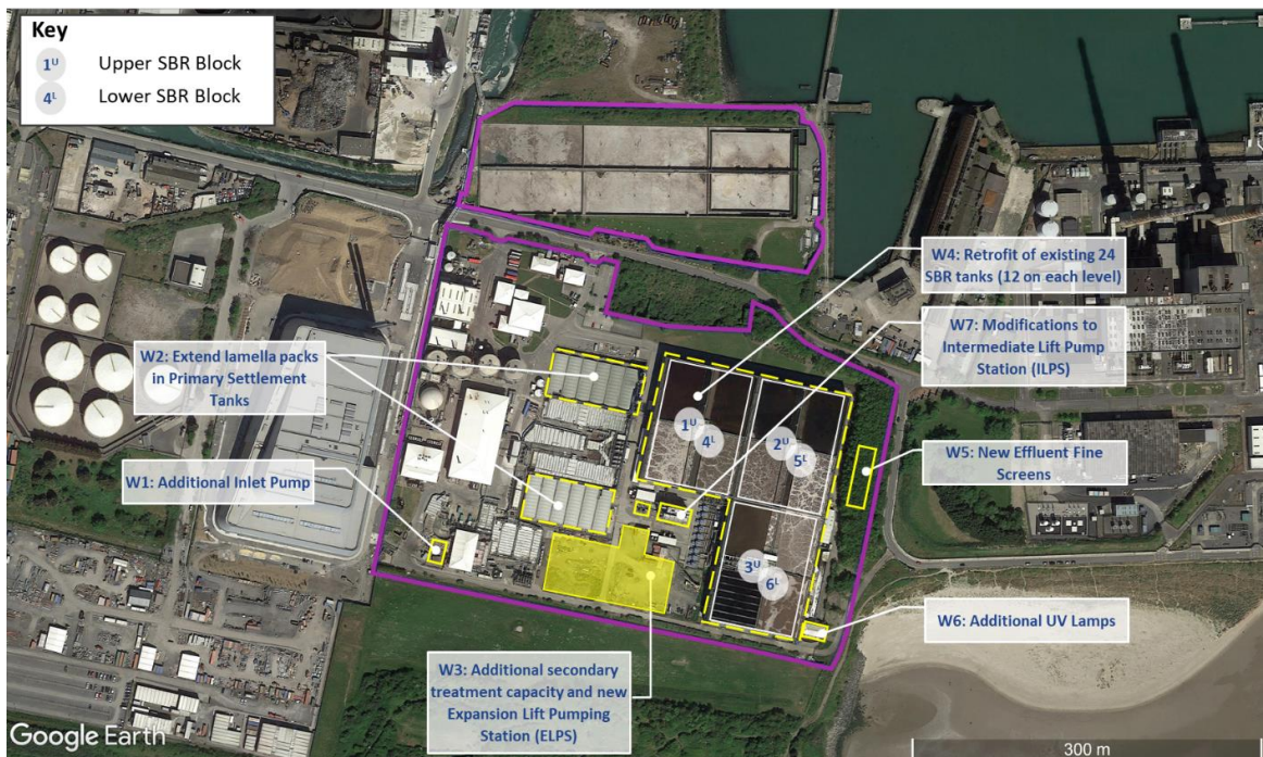
Figure 25: The Proposed Upgrade Project – Wastewater Stream Upgrades (Source: Figure 3-6 of the EIAR)
