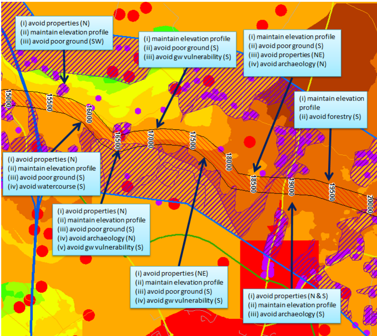
Figure 1-14 – Typical example of decision making process adopted in defining the ‘Preliminary 200m Pipeline Corridor’
